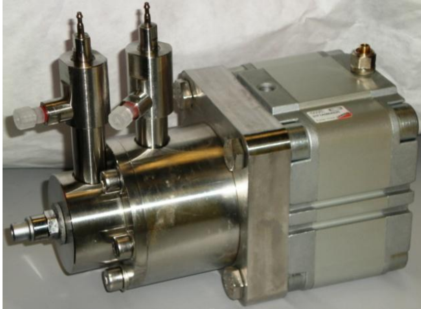
Figure 1. Component of the perfusion bioreactor applying hydrostatic pressure cycles (culture chamber, pneumatic actuator and hydraulic valves), not yet connected to other components.
